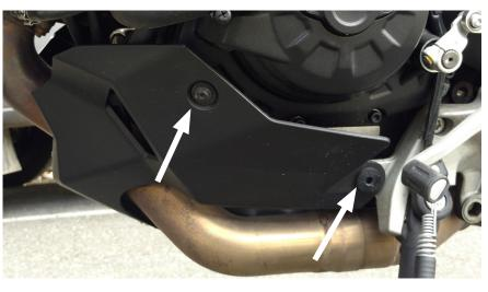
(2) Remove left side attachments. 4mm and 5mm allen wrenches.
