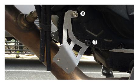
Install left bracket as shown. Replace upper OEM screw with supplied stainless M6x35 screw. (A) Torque to 8 Nm. Use OEM screw in lower position (B) Torque to 10 Nm.
