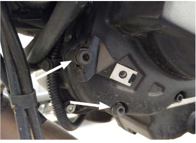
Remove two screws from left side, 5mm allen tool. Remove small black bracket.
