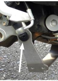
(1) Install rear bracket. Use OEM large head aluminum fasteners.
