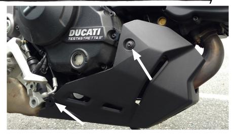
Remove right side attachments. 4mm and 5mm allen wrenches.
