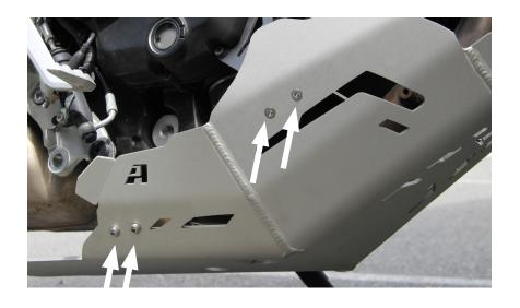
Loosely install right side screws. 2x M6 button head at rear, 2X M5 flat head at front. Use a drop of loctite on each screw.
