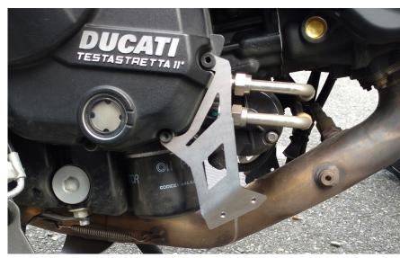
(5) Install Altrider bracket as shown, re-use OEM screws. Torque to 10 Nm.
