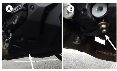
(A) Remove bottom screww, M6 allen wrench.
