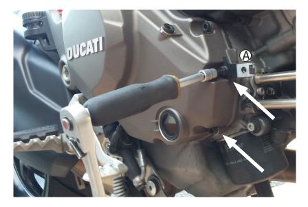
5mm allen wrench, remove 2 screws shown, remove small black bracket (A)
