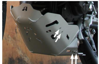
Loosely install left ide screws. 2x M6 button head at rear, 2X M5 flat head at front. Use loctite. Progressively tighten all 8 screws on the skid to final torque, working on each screw in turn for even installation. M5 screws to 4.3 Nm. M6 ot 8.5 Nm.
