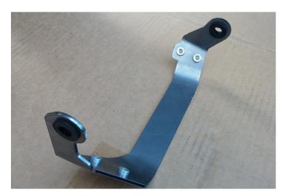
Remove rubber grommets from OEM belly pan. Insert into altrider bracket. (HINT: use small amount of water to lubricate rubber and make insertion easier).
